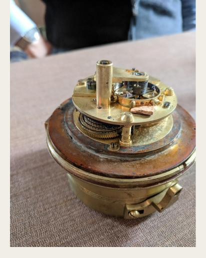
The interior of Simon Willard's marine chronometer at Willard House and Clock Museum, showing balance wheel and helical hair spring held in place by a small piece of cork--a means of protecting the delicate balance pivots while the movement is at rest.
