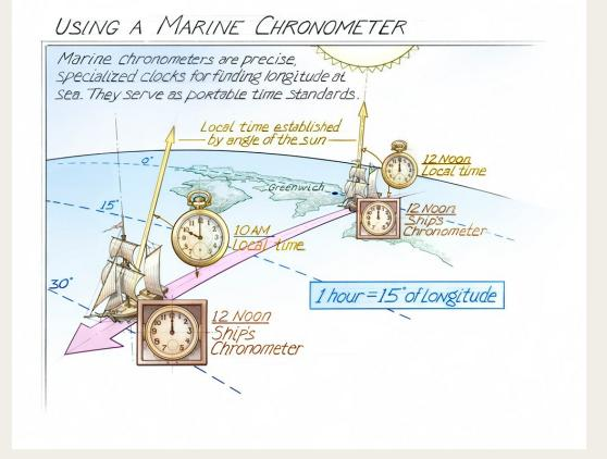
"Using a Marine Chronometer" graphic which demonstrates how a marine chronometer was an integral tool in finding one's location on the open ocean. Image from Time and Navigation, an exhibition at the National Air and Space Museum. Courtesy Smithsonian National Air and Space Museum (NASM9A11818).
