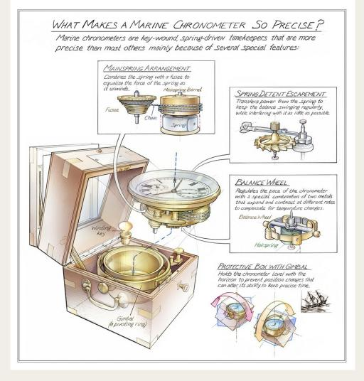
"What Makes a Chronometer so Precise?" graphic which explains the key features of a marine chronometer. Image from Time and Navigation, an exhibition at the Smithsonian National Air and Space Museum. Courtesy Smithsonian National Air and Space Museum (NASM9A11805).
